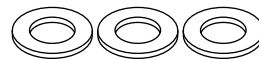
Upper-to-Lower Mount Hardware (3x) 3/8" x 3/4" Bolts (3x) 3/8" Split Lock Washers (3x) 3/8" Flat Washers
